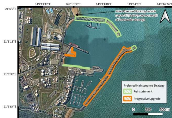
Figure 89 Plan of Port of Mackay showing reinstatement and progressive upgrade as the recommended maintenance strategies for their respective structures.
