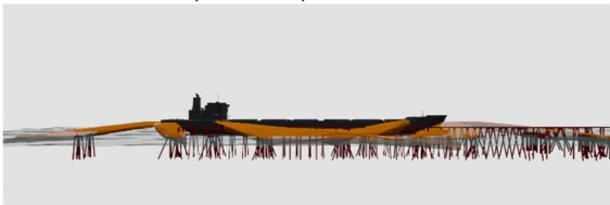
Figure 24 A visualisation of the envelope snapback paths for a capsized vessel in ballast high-tide conditions.
