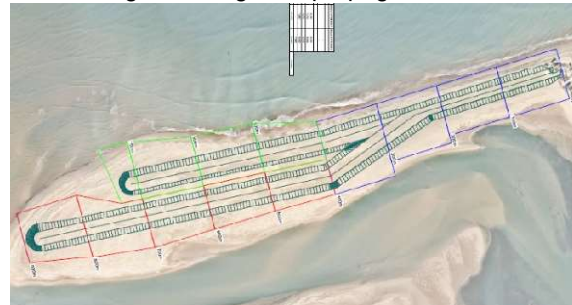
Figure 83 Preliminary dune design depicting the alignment and structure of the foredune and primary dune to provide suitable protection. Source: BMT
