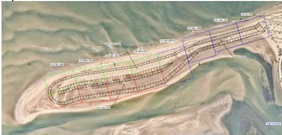
Figure 84 Detailed dune design depicting the alignment and structure of the foredune and primary dune to provide additional volume. Source: BMT
