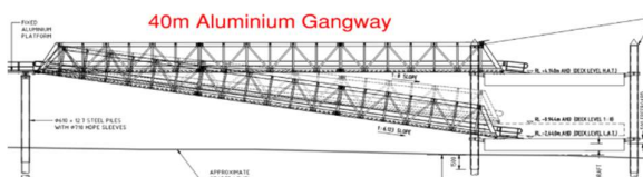
Figure 1: Tender design with two short gangways and a floating mid-landing platform resting on a stop frame.
