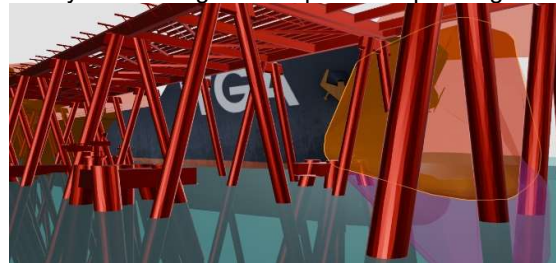
Figure 25 A visualisation of the snapback path of a forward breast line that has parted near the winch. Though the snapback barriers on the dolphin were modelled, the orange path (which is a truncated wavefront based on time to clash detection with the structure) shows a line that was able to effectively whip sideways around the barrier and get halfway under the deck before hitting the water level. The untruncated path is shown in purple.
