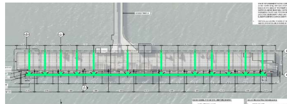
Fig 4 - Plan illustrating the new fender beam and prop locations.
