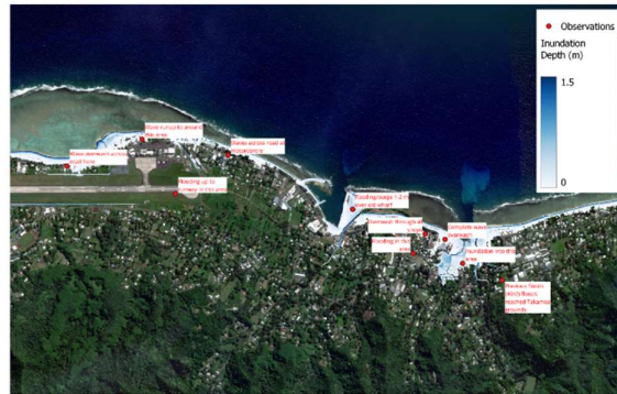
Figure 64 Coastal flooding on the north coast of Rarotonga due to the passage of Cyclone Sally (1986). The inundation levels are compared against observations providing confidence in the model performance.
