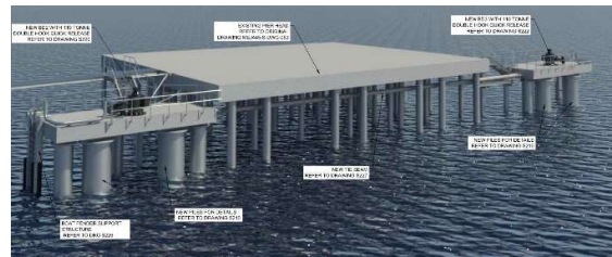
Figure 50 Isometric View of New Spring Mooring Dolphins
