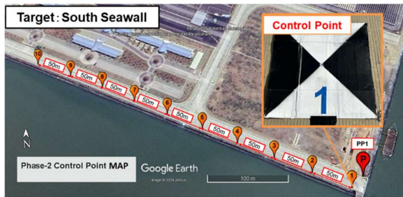
Figure 75 Control points arrangement
