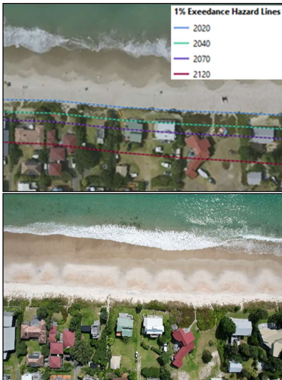
Figure 113 Current 1% exceedance hazard lines (top pane) vs coastal erosion line after cyclones Hale and Gabrielle (bottom pane) - WP5
