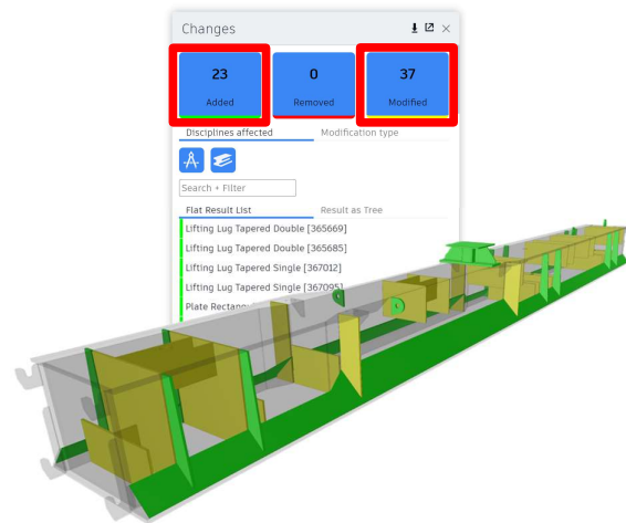
Figure 129. Automated model change detection for a jetty headstock assembly. The Common Data environment is used to detect changes between work-in-progress design model versions by identifying elements that have been added, removed, or modified. Automation of this task creates capacity for delivery personnel to investigate creative opportunities to mitigate design quantity growth. (Source: McConnell Dowell).
