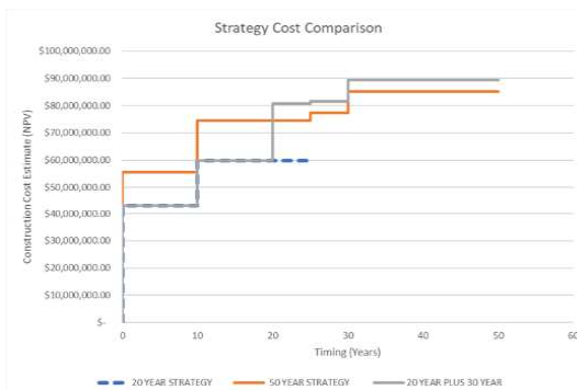
Figure 53 Cost estimates for each strategy, expressed in net present costs assuming 4% discount rate. (Source [1])
