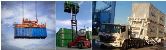
Figure 2. Twinlift Handling Equipment for Empty Container
