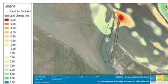
Figure 47 Bed level difference plot results for Scenario 2
